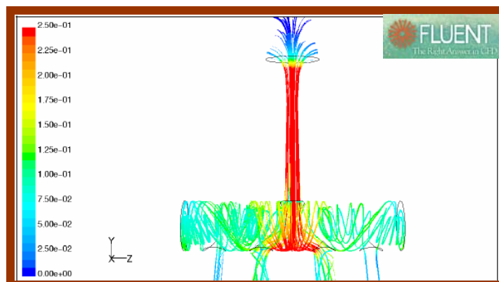
CFD model of Intake and Plenum
